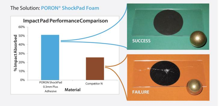
As you can see in the graph above, **PORON ShockPad Foam absorbs twice as much force as equivalent competitive material** in real-life drop conditions.
